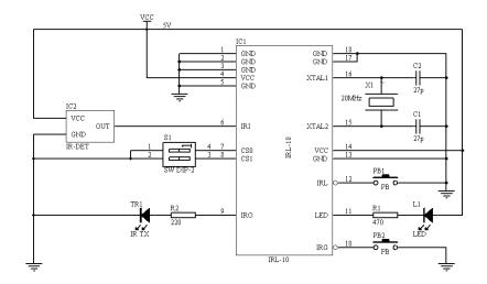
Infra red detector IC2 receives 37-40KHz modulated IR signal from common remote control emitters and produces a demodulated signal corresponding to the envelop of the IR signal. Such as PIC26043SM by Kodenshi available from Farnell part no. 139-877
